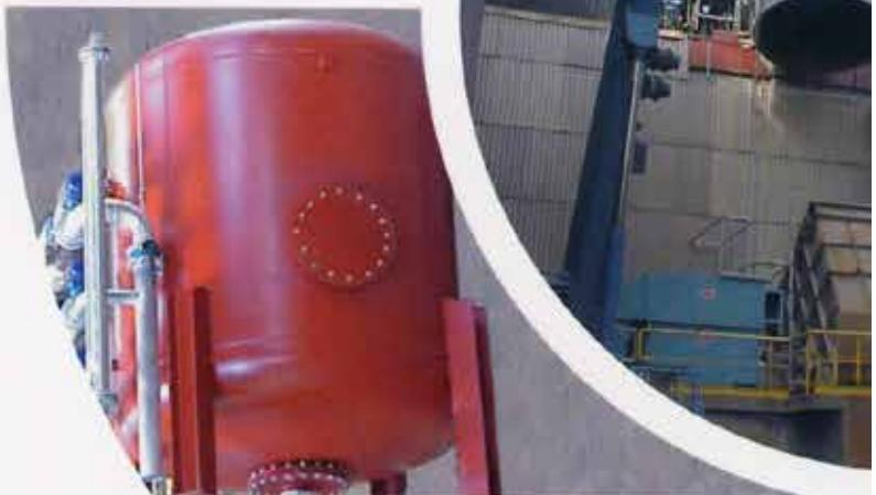
■ We also produce all the collars for such parts. Our rolling machine's maximum capacity is 3m for a thickness of 12mm (standard or conical collars).
